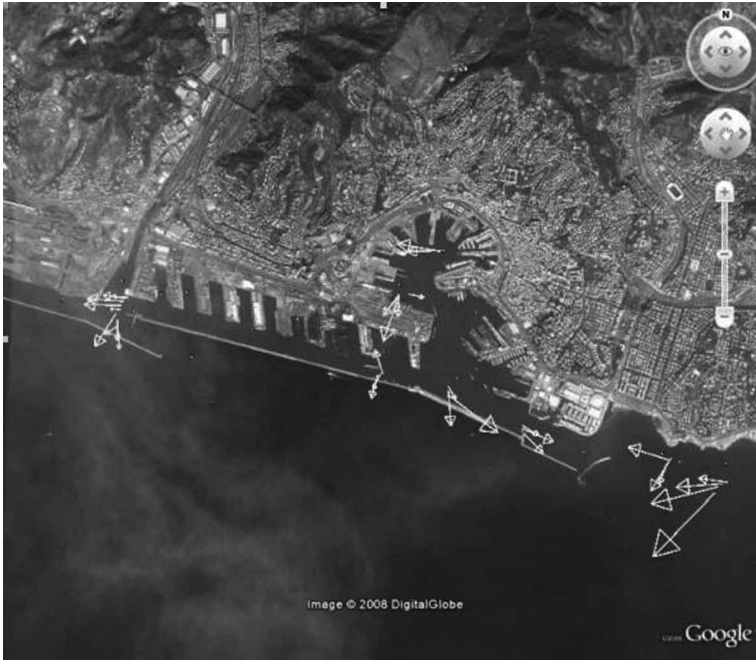
Figure 2. Surface current vectors obtained from the ADCP measurements (beginning of March campaign, characterised by a strong wind swinging from north-east to north): vectors, magnified only for graphic reasons, are proportional to the intensity (with the highest values of 50 \text{ cm} \cdot \text{s}^{-1} ) and direction of the current (from Google Earth, 5.0.11337.1968 (beta ver.)).
