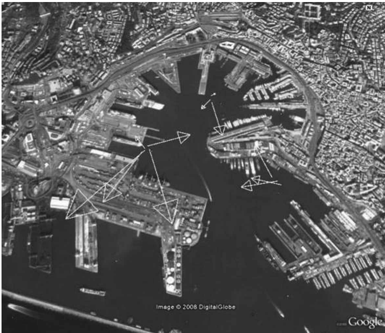
Figure 3. The dock: vectors of the surface current obtained from the ADCP measurements (end of March campaign, with strong wind from south-east): the dimensions are proportional to the intensity (with higher values of 25 \text{ cm} \cdot \text{s}^{-1} for the largest vector) and direction of the current (from Google Earth, 5.0.11337.1968 (beta ver.)).
